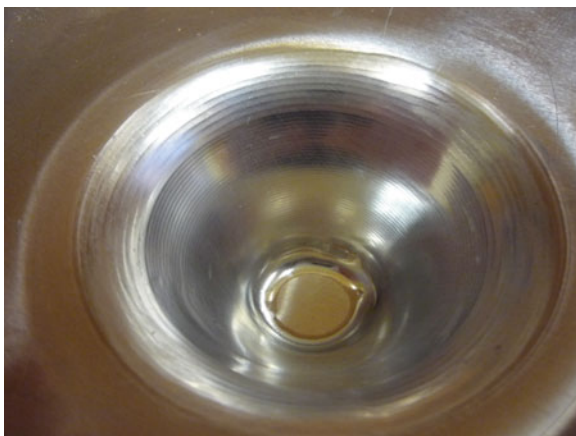
Fig. 19 Photo of the formed part with local thinning at the beginning of the forming (2 test)
